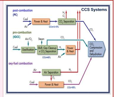
include high pressure membrane filtration, adsorption/ desorption processes and cryogenic separation. Precombustion removal is done through gasification which combines coal with steam and oxygen to produce "syngas" - a mixture of carbon monoxide and hydrogen. After the CO<sup>2</sup> is captured, it is injected into the ground in oil or gas fields for reuse in enhanced fuel recovery.
